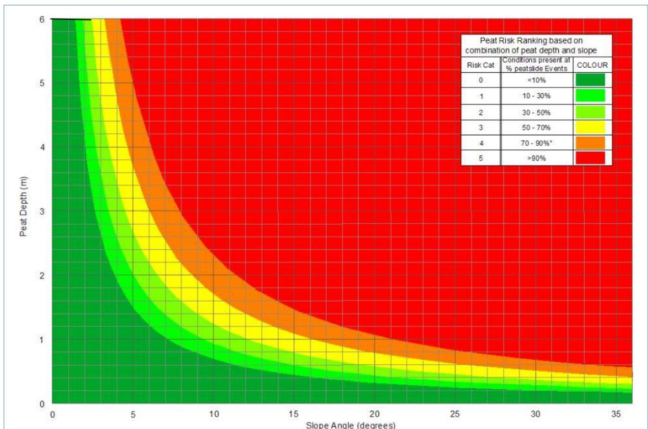
Figure 2-8 - Relationship of Depth and Slope to Peat Slide Events
