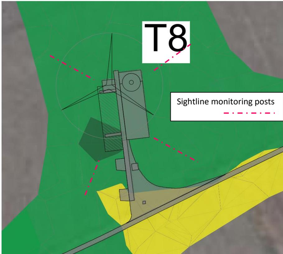
Figure 3-1 Example of a typical monitoring post layout
