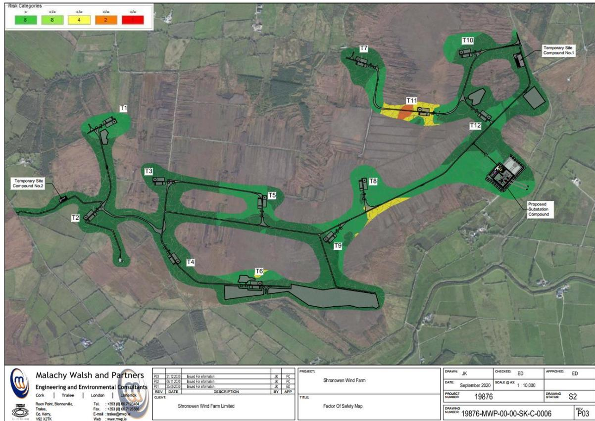
Figure 2-12: Factor of Safety for Peat Stability across the study area with 10kPa surcharge applied (Unmitigated)
